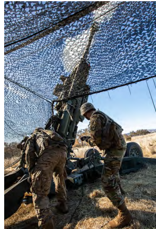
CDT Citroen pulls the lanyard of the M777 Howitzer, sending a 155mm round several kilometers away into the impact area.
